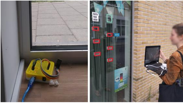
Figure 6. DoS 6: Receiver of polling devices connected to mini computer behind the window (left) and researcher with laptop and base station (right) to update the displays.
